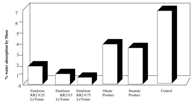
Fig 1. Reduction of Water Absorption
