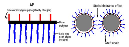
Error! Schematic picture of acrylic polymer (AP) and the related steric hindrance effect on the dispersion of cement particles
